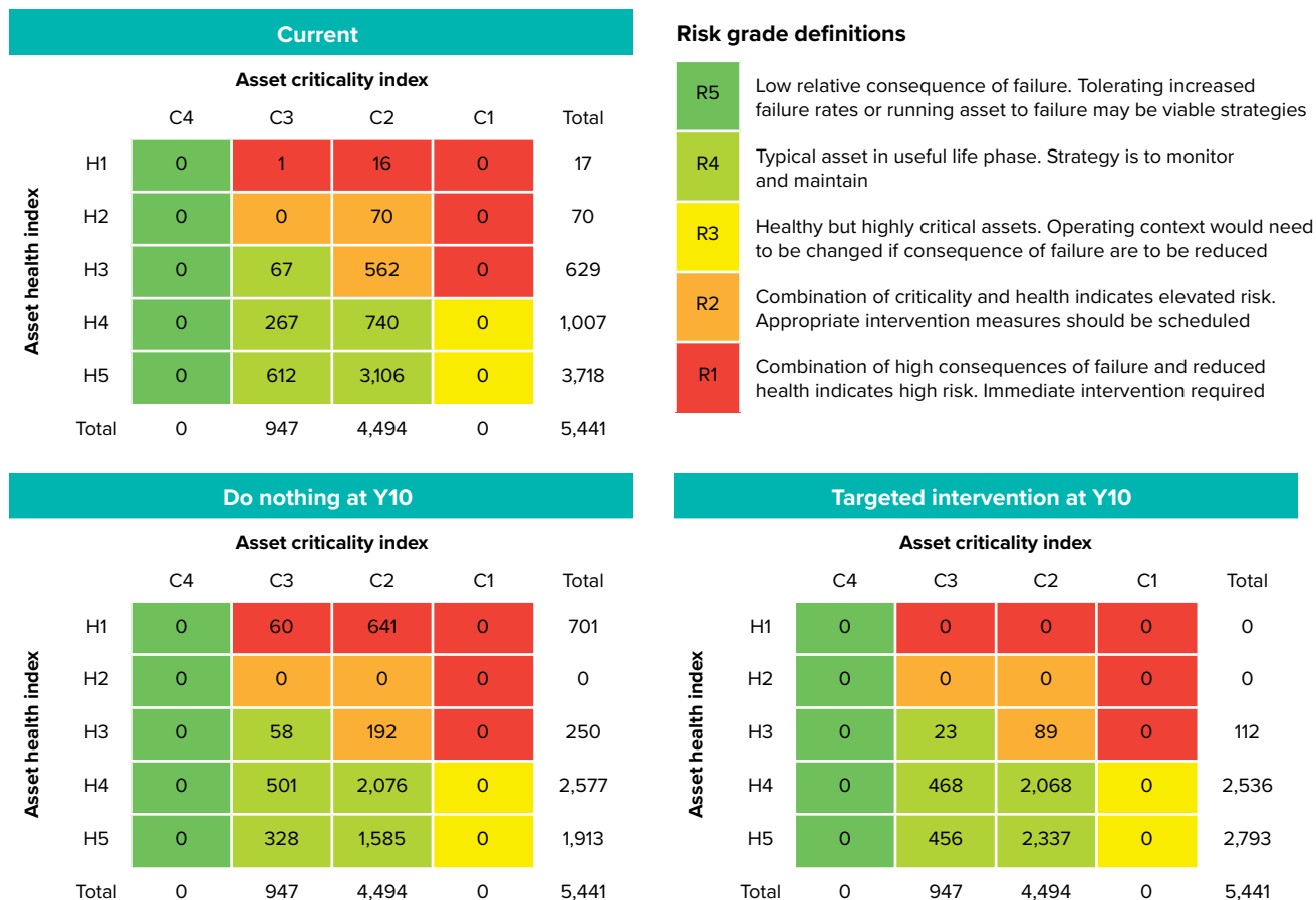
Figure 7.4.6 Subtransmission pole risk matrix
